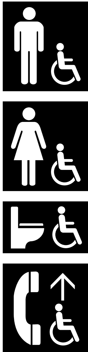
Figure 13 Examples of service identification signs incorporating the International Pictogram of Access (See Clauses 4.6.7 and 6.3.1.1. )
