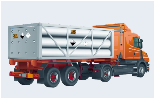
Figure 3: Truck hauling multiple element gas containers (MEGCs)
